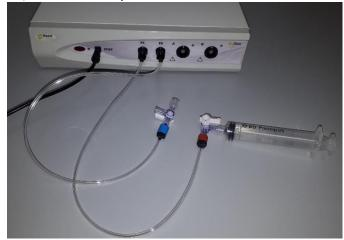
Next the probe is directly connected on the back of the tap.
